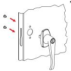
1. Place the locking handle (Ref. No. 10) on the right hand door and fasten with two #8-32 X 1/4 hex-head bolts and lock washers, provided with the handle.
