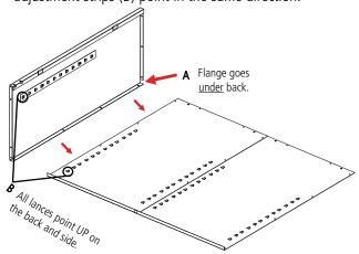
**4.** Attach the top (Ref. No. 8) to the unit by sliding the outer flange over the back of the unit and the side flange to the side panel on the unit. The threaded studs should go
