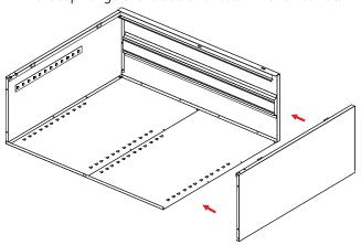
**6.** Attach the sill (Ref. No. 4) to the sides. Place a nut (Ref. No. 19) loosely on each of the studs and slide the ends of the sill into the slots on both sides of the unit. Then, securely tighten the nuts.
