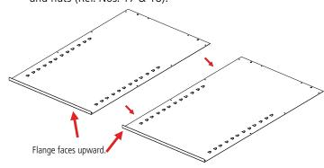
**3.** Attach the left side (Ref. No. 2) to the back by placing flange (A) around the back and bolting tightly together with four bolts and nuts. Be sure that the lances on all the shelf adjustment strips (B) point in the same direction.
