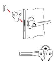
With the handle still in the open position, hook the locking bars (Ref. No. 9) to the locking cam (see "A" at left). Once in position, slowly rotate the door handle to the closed position so the lock bars prot rude from the holes at the top and bottom of the door (shown at right, below).
