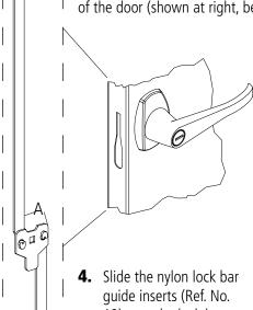
Guide the nylon lock bar guide inserts (Ref. No. 12) over the lock bar ends and through the door slots (see "B" at right). Push down firmly until the guides snap into place.
